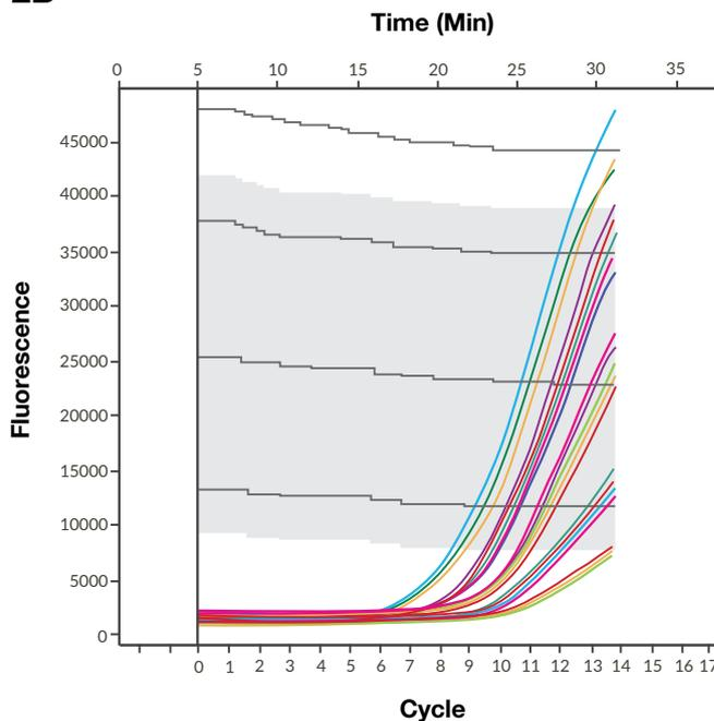
Figure 2B. Example of real-time high fidelity amplification of multiple libraries. 20 libraries, spanning a ~64-fold concentration range (6 cycles), were simultaneously amplified and terminated after 14 cycles. 14 of the 20 libraries fall within the targeted amplification range. The remaining 6 libraries could either be used as-is, noting that they may be outside the optimal concentration range, or they could be re-amplified individually or in high- or low-concentration groups.
