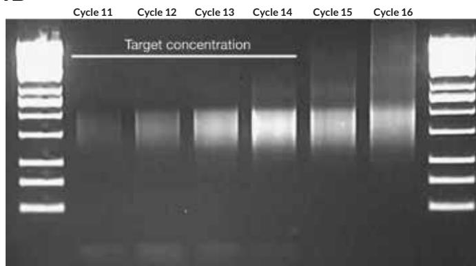
Figure 1B. Gel image of a typical library stopped at different amplification cycles. Low and high molecular weight artifacts increase progressively with additional cycles.
