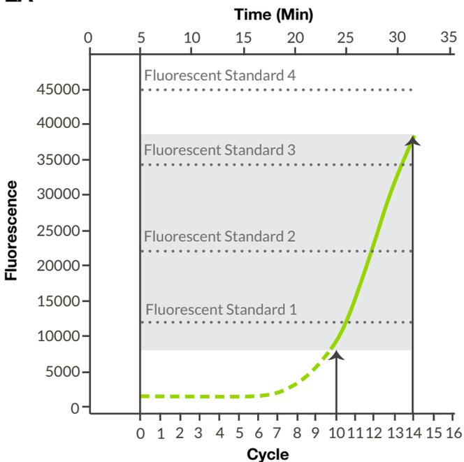
Figure 2A. Superimposed amplification plots for reactions terminated at the lower bound (hashed line, cycle 10) or upper bound (solid line, cycle 14) of the targeted concentration range (grey box). Library amplification reactions should ideally be terminated anywhere within the indicated target concentration range.
