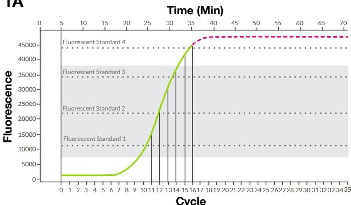
Figure 1A. Libraries are amplified using a SYBR® Green-based real-time, high-fidelity PCR master mix. Four triplicate wells of the PCR plate contain fluorescent reference standards representing a range of distinct DNA concentrations. Reactions terminated between Standards 1 and 3 represent the optimal library amplification range (grey box), depicted here from cycle 10 – 14.
